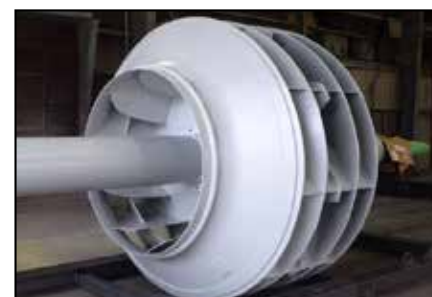
Dynamically balanced ARC S7 AR coated fan.
