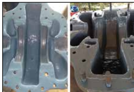
Repair being performed, body and cover.
