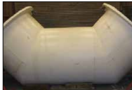
Exhaust elbow in shop laydown.
