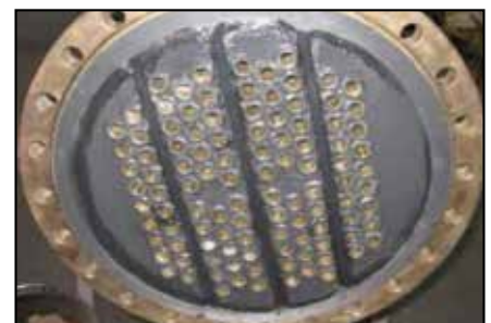
Completed tube sheet.
