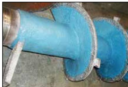
ARC MX1 applied and tips welded.
