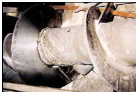
Abraded screw conveyor.
