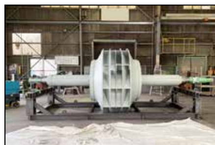
ID Fan in paint shop.
