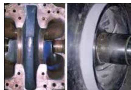
Coated sections of pump.
